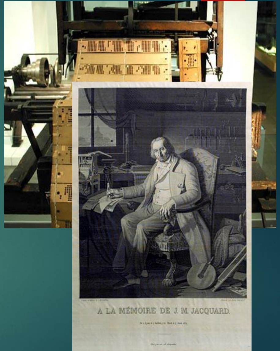
Image of Jacquard woven in silk with a Jacquard Loom; required 24,000 punch cards (1839)
